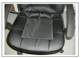
Place the COS onto the chair seat so that the maximum weight of the chair occupant is directly over the sensor.
