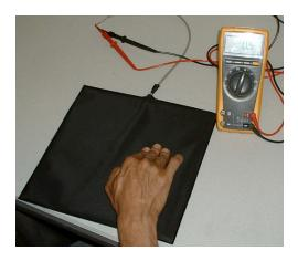
When the sensor is activated the reading should be less than 10 ohms. In this picture the resistance indicated as the sensor is activated is 0.5 ohms, which is less than 10 ohms, indicating a functional sensor.
