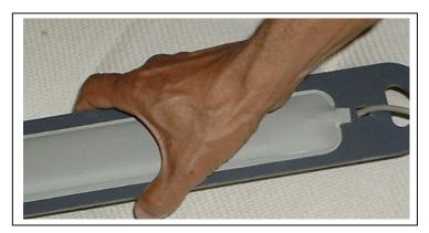
Shown here is the correct way to remove the BOS from the bed. Grasp the sensor carrier and remove the sensor without pulling on the wire.
