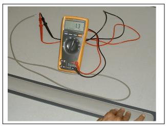
In testing the sensor, be sure to activate it in multiple positions as shown above left, middle and right.
