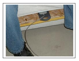
When placing the sensor be sure to have the wire exit the bed opposite the patient bed exit. Shown in this photo is the WRONG orientation for the bed sensor. Having the wire exit directly under a person's feet will encourage tripping and potential premature failure of the sensor due to accidental pulls on the wire.
