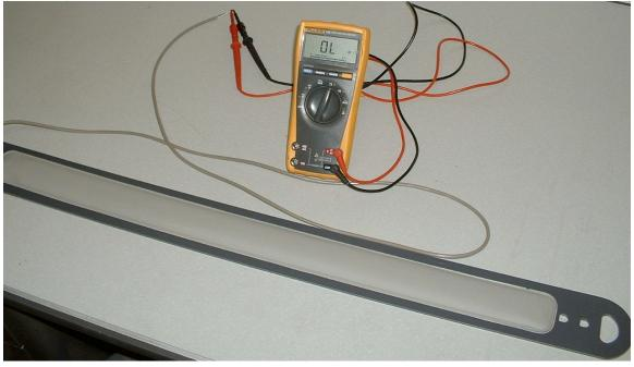
In the pictured test the resistance meter is reading beyond its capability to record a resistance reading. Interpret this as much greater than 10 Mohms.
