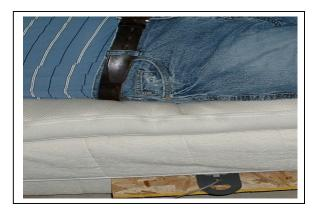
Position the BOS so that the person's weight is centered on the sensor. In general the best position for the sensor is under the buttocks or shoulders. In either case the sensor must be on a firm flat surface.
